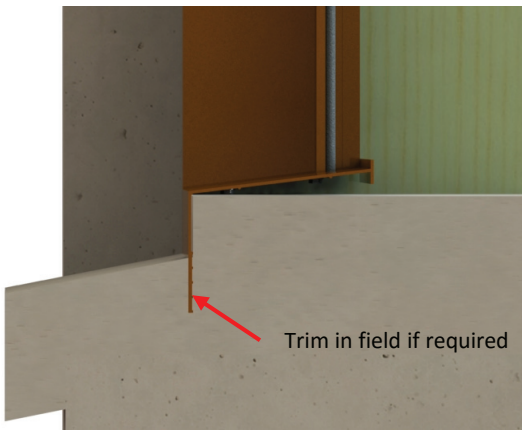
Sill cross section view
